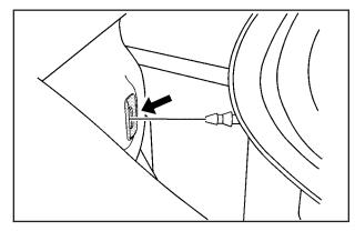
When you reinstall the headlamp assembly, make sure to line up the pin in the headlamp assembly with the slot in the vehicle.
